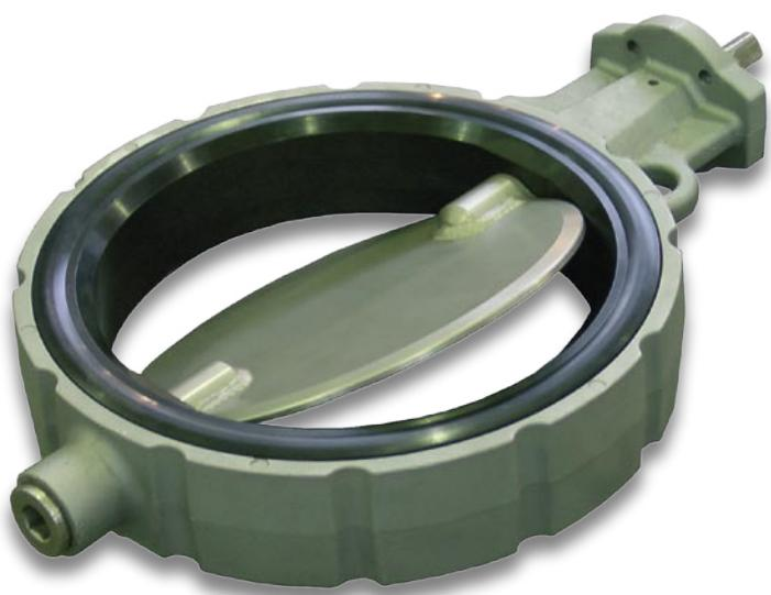
**VW Butterfly Valves** consist of a single block body manufactured from die-cast aluminium, a carbon 304 stainless steel disc including shafts and an elastomer seal.
