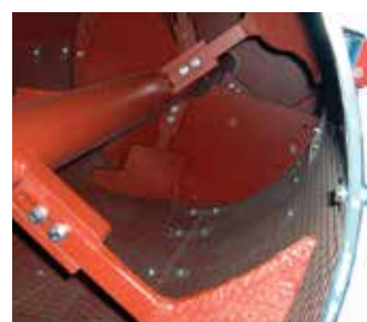
Anti-wear tool coating and chamber lining
